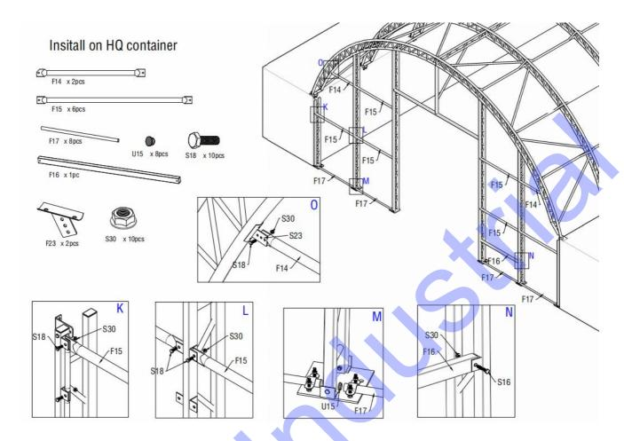
As Above Figures shows, find out all spare parts for the front wall. connect them together by use screw, make sure the spacing. There are stake pegs for base plates.
