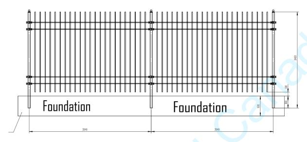
Plug the posts into the foundation 500mm as shown
